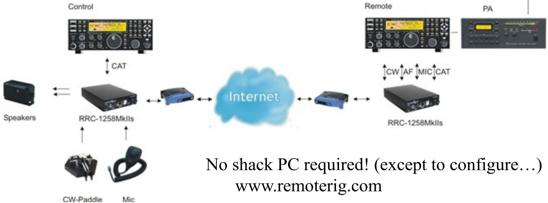
Uses a pair of RemoteRig “modems” to send audio and control signals to radio.
