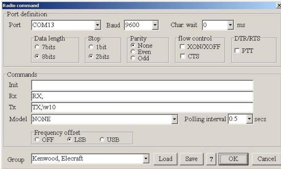
In the Fldigi program this is done in the tab for “Configure/Rig/Hamlib” or the tab for “Configure/Rig/RigCAT.” The Fldigi settings are shown here:
