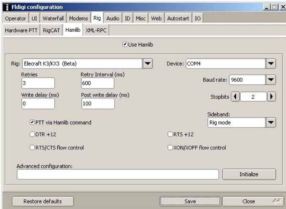
You only need to minimally setup for Transmit (TX), and Return to Receive (RX), for the radio type of an Elecraft K3, which uses the Kenwood command set. Other control functions and radio commands may also be controlled through the RHR Helper App for Chrome such as controlling and logging the radio's frequency.
